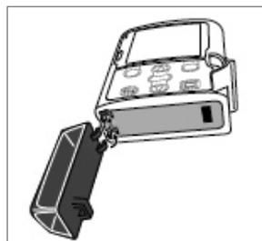
Figure 3: Inserting cassette hooks
