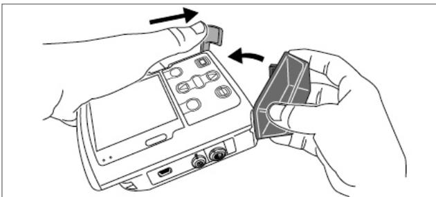
Figure 17: Removing the cassette
