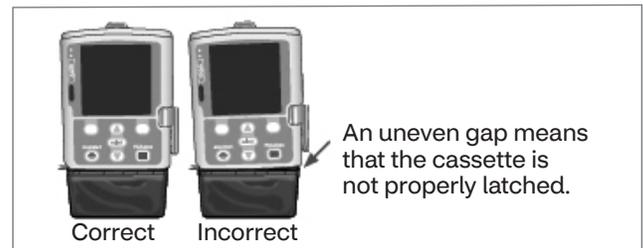
Figure 5: Attaching the cassette
